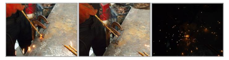
Striking an arc took a couple of tries, but once I figured out the correct distance and angle
