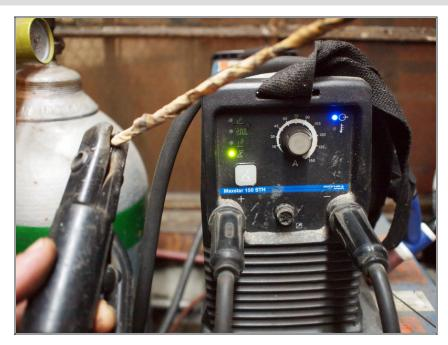
I used the recommended settings for a 3/32 (ish) rod -- DCEP, around 100 amps.
