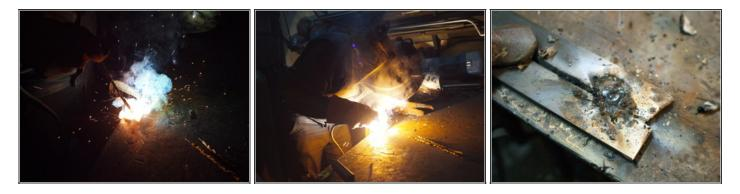
Totally welding with home-made electrode. Splattery and ugly (you can partially blame user error and a little bit of a learning curve) but definitely looks like a weld.
