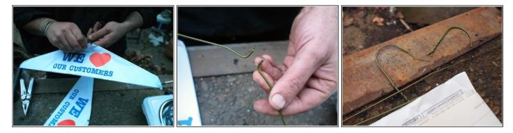
• Straighten the hanger, then cut pieces of welding-rod size: about a foot long will work.
