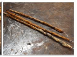
Bake the rods. This drives out moisture, and also makes a carbonized shell that keeps the
