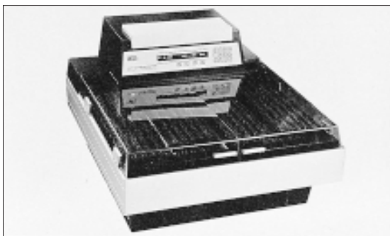
Fig. 2.2 Gamma counting in the eighties. 1277 GammaMaster featured a staggered array of 1.5 inch through-hole detectors and RiaCalc software.
